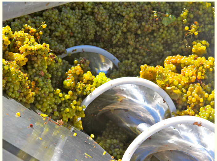
California Zinfandel is ready to pick, while the crusher destemmer goes into action on Chardonnay grapes.
